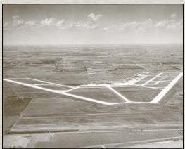
southeast direction will accommodate all traffic on the airport for 97 per cent of flying weather. Aircraft landing and taking off under high velocity east and west winds, which may occur as much as three per cent of the time, will be accommodated through the use of a short east-west runway.
